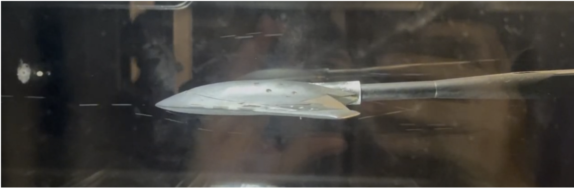
Figure 12: Helium Bubble flow for flap down wingtip configuration at Angle of Attack of -4 Degrees
