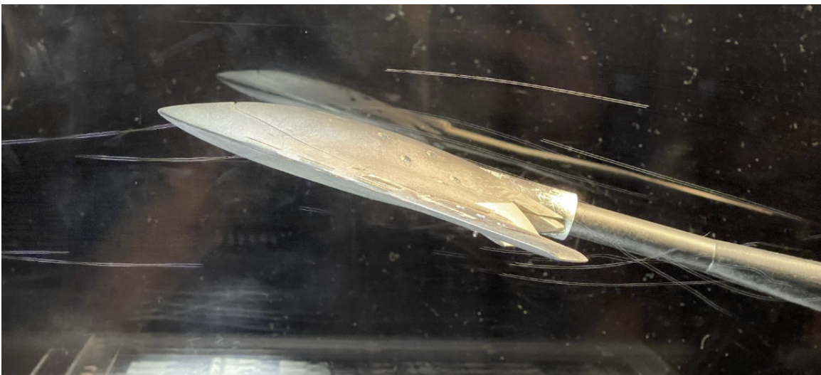
Figure 14: Helium Bubble flow for flap down wingtip configuration at Angle of Attack of 14 Degrees
