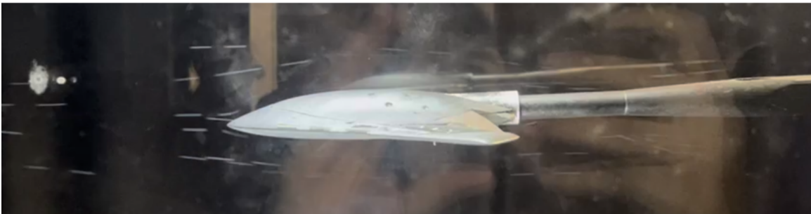
Figure 13: Helium Bubble flow for flap down wingtip configuration at Angle of Attack of 0 Degrees
